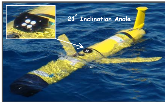
Fig.1. Slocum Coastal Glider equipped with an irradiance sensor (OCR-504I).
